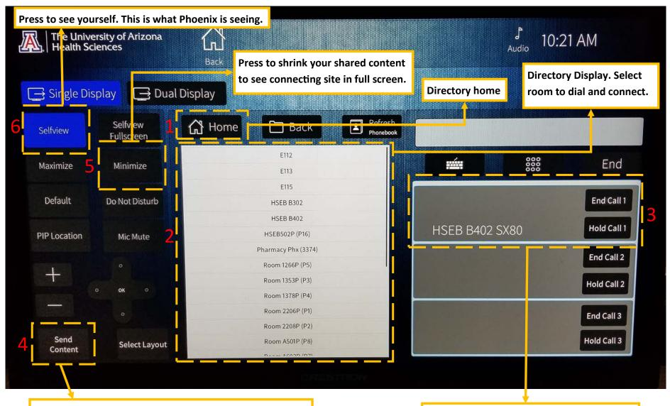
Press to send content to connecting site from the in-room computer or other device (i.e. laptop, doc cam, etc.)
